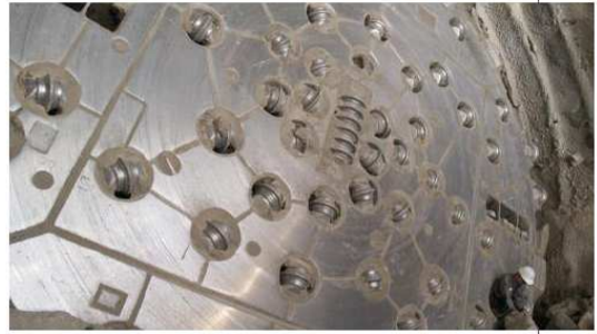
Above left: Breakthrough of an 8.16-m Wirth EPB TBM equipped with TunnelTec tools on the Castellanza metro project, Italy. The cutterhead is equipped with both static rippers and scrapers and disc cutters with carbide bullet inserts. Right: Disc cutters shown on the cutterhead of a 9.90m-diameter NFM Technologies TBM on completion of 1140m in a single month for the Madrid-Gijon high-speed railway route
